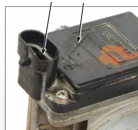
Cracked Plastic Connector and Housing
